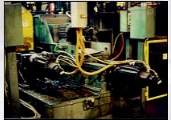
Servo Upgrade System replaces AC motors and gear box transmissions on over 100 transfer line stations.
