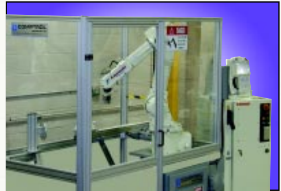
Manufacturing Work Cell with 6-axis robotic part interpolator and pneumatic feed slide.
