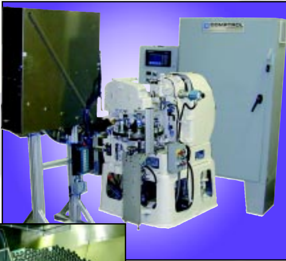
Automatic Loading & Part Orientation System included gravity fed magazine loader, lift and rotate orientation station, operator interface, and control system.
