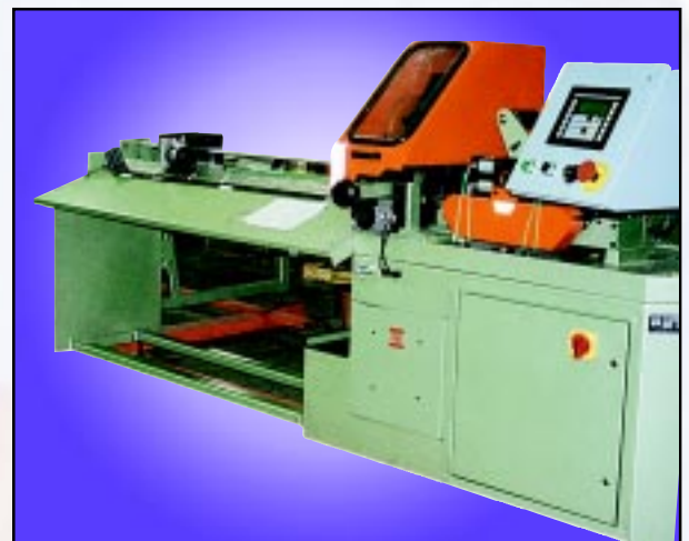
Programmable Positioning Stop Retrofit Package with new operator interface and controls for cut-to-length application.
