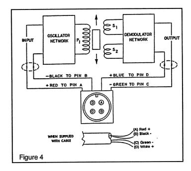
With Comptrol LVDTs, the input and output circuits are electrically isolated from each other and from the mechanical structure of the tensioncell. Thus, they may be used in "floating ground" or "ground return" systems. This eliminates the need for extra circuit boards which are required for most straingage loadcells.
