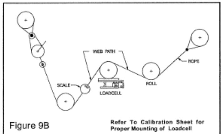
4. Repeat Step 3 for the loadcell mounted on the opposite end of the measuring roll.
