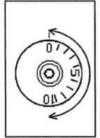
NOTE: Rotating the dial beyond the "0" or "10" markings on the scale has no effect on the damper adjustment.
