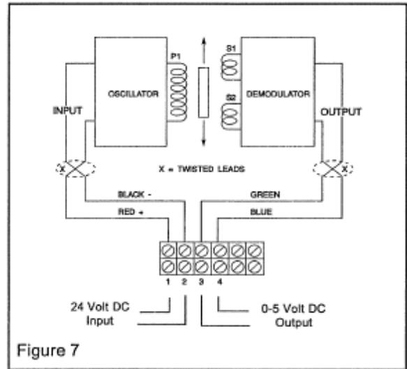
4. Measure the output voltage of the LVDT between the Green and Blue leads with a voltmeter with a sensitivity of at least 100,000 ohms per volt. The output voltage should be between zero.
