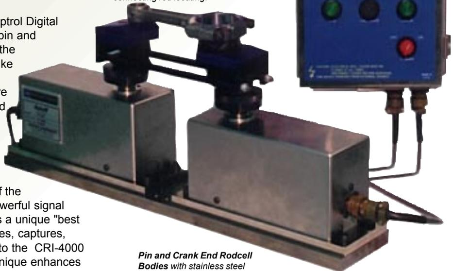
*Pin and Crank End Rodcell Bodies with stainless steel covers house microprocessor electronic*
