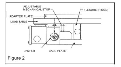
The Model DH151 is designed for application where the resultant strip tension force components cause the Monocell Load Table to deflect toward the Base Plate. The deflection of the Load Table toward the Base Plate caused by the tare and strip tension forces is defined as the "Compression Mode". The small tare force component can be zeroed out by following the Electrical Zero Adjustment procedure outlined later in this bulletin.
