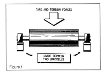
The Model DK151 is designed for applications where the resultant strip tension forces cause the Load Plate to deflect away from the Base Plate. The deflection of the Load Table away from the Base Plate is defined as the "Tension Mode". In these cases, the centerline of the roll is to the right of the pivot point of the Comptrol "C" Flexure. The small force created by the tare weight of the roll is then in the tension mode.
