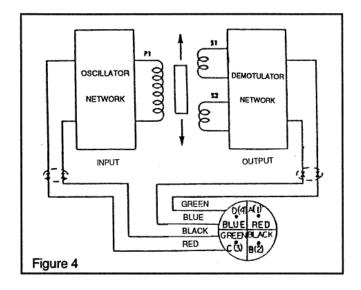
Because of this, the use of a "well regulated" constant voltage power supply is essential for accurate and repeatable tension measurement.
