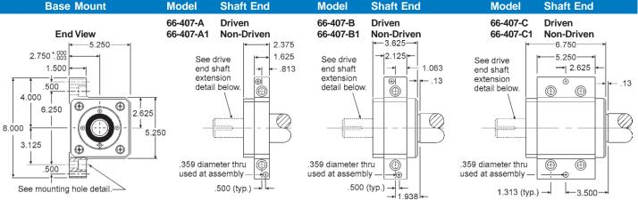
Note: For each Type A or A1 bearing block required, add .250" to ballscrew thread length.
